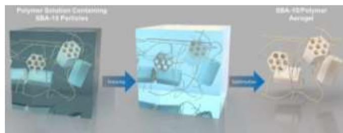
**Figure 2.** Schematic representation of the freeze-drying process to form hybrid aerogels.
